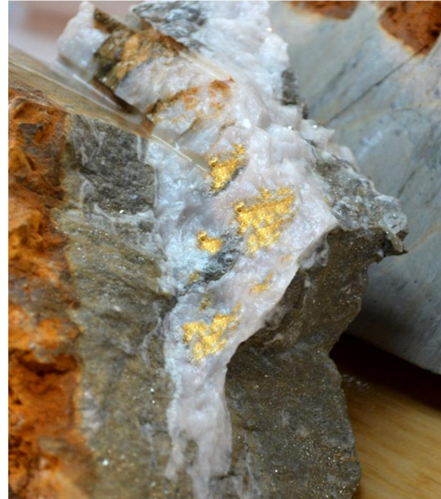
Photo of coarse visible gold in a quartz vein channel sample, Trench 3 – Croteau Bouchard Shear Zone, Croteau property. Grab sample assay, 92.57 g/t gold: channel sample average assay, 14.37 g/t Au/7.5 m.
