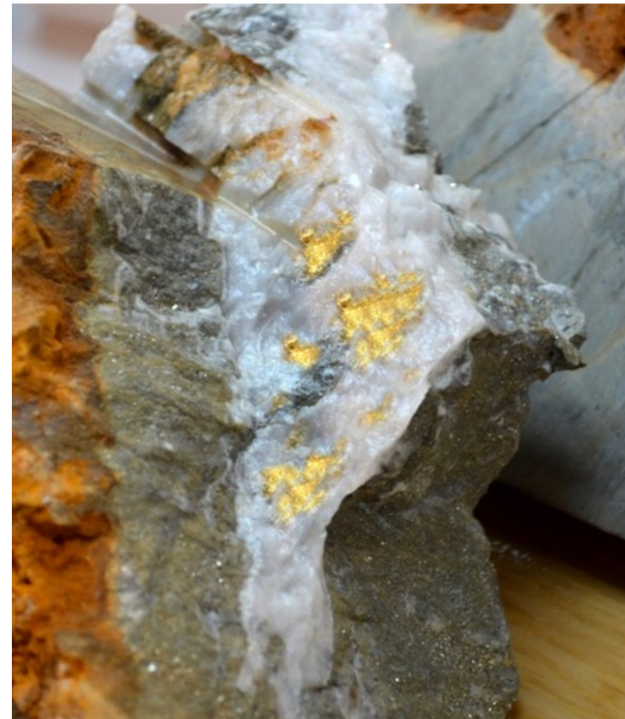
Photo of coarse visible gold in a quartz vein channel sample, Trench 3 – Croteau Bouchard Shear Zone, Croteau Est property. Grab sample assay, 92.57 g/t gold: channel sample average assay, 14.37 g/t Au/7.5 m.
