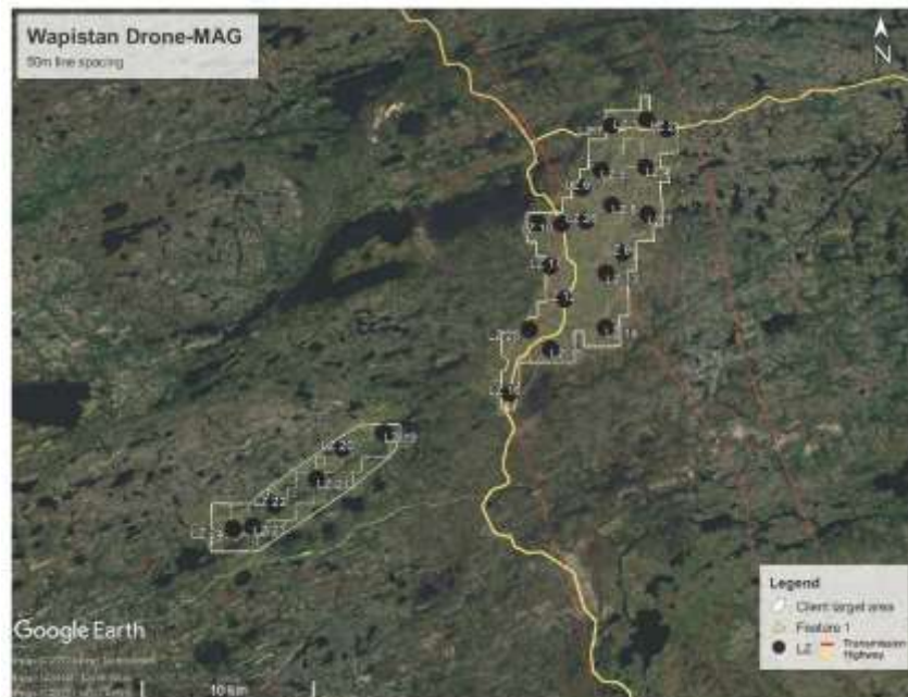
Figure 2: Area covered by the current, high-resolution UAV, drone supported magnetic survey. The survey includes 2,450 line kms flown between 15- 30m above ground level. The area is easily accessible by highway with hydro lines either crossing the property or in proximity to it.
